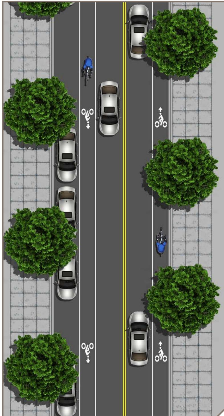
Standard Bike Lane Schematic Layout with (left side) and without (right side) On-Street Parking
