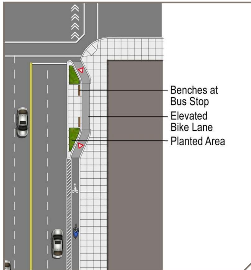
Special accommodations should be considered at bus stops. This conceptual schematic layout shows how a bike lane can be integrated into a bus stop area
