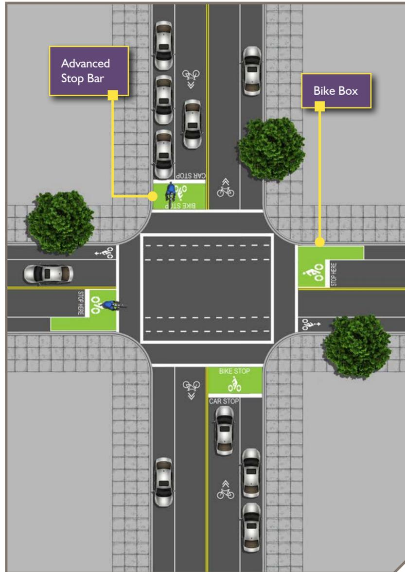
Schematic Layout for a Bike Box and Advanced Stop Bar
