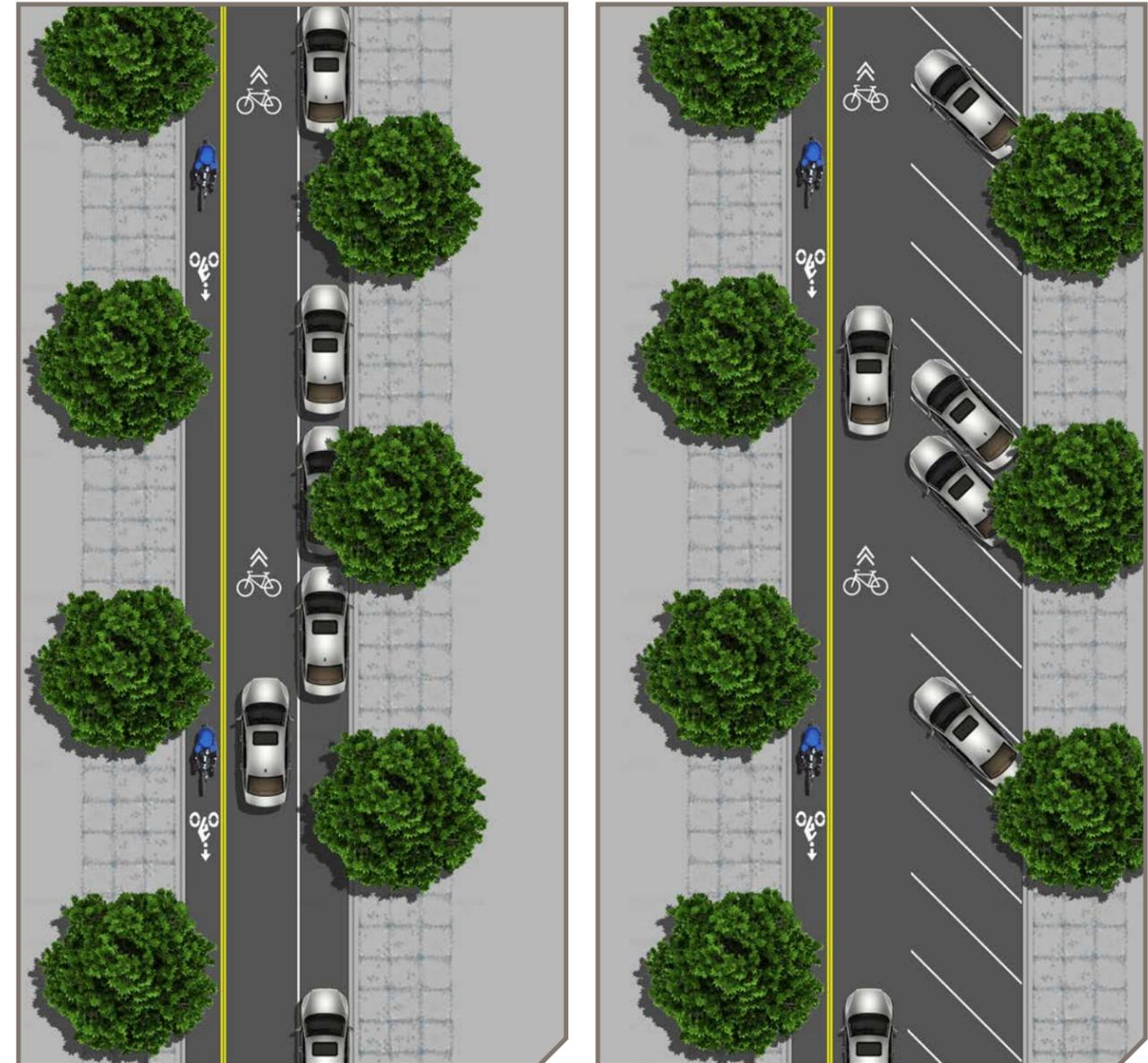
Contraflow Bike Lane Schematic Layouts with alternative parking configurations. Diagonal parking can be used if there is adequate width to mitigate for lost parking on the left side of one way streets
