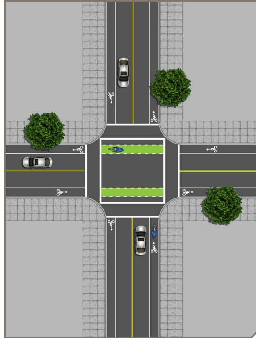
Schematic Layout using green paint for a Bike Lane Continuation
