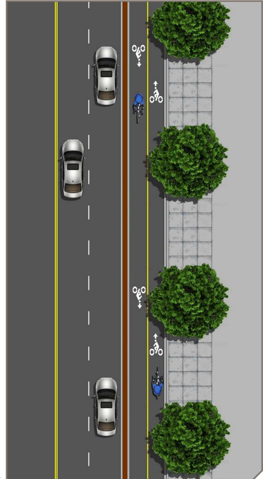
Cycletrack schematic layout using a monolithic separation between bicycle and motor vehicle lanes
