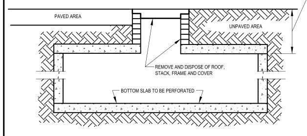
NOTE: ABANDONED MANHOLES, INLETS, AND/ OR VAULTS SHALL BE BACKFILLED AND PAVED IN ACCORDANCE WITH STANDARD PLATES NO. BC 576.18, BC 576.19, AND BC 576.20
