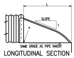
\* INVERT ELEVATION TO BE AT THE PIPE END OF THE STANDARD END SECTION. ELEVATIONS TO BE NOTED ON CONSTRUCTION PLANS.
