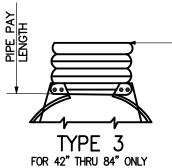
INCLUDES ONE FOOT OF PIPE LENGTH AS A CONNECTOR SECTION. THE CONNECTOR SECTION WILL BE ATTACHED TO THE END SECTION BY GALVANIZED RIVETS OR BOLTS.
