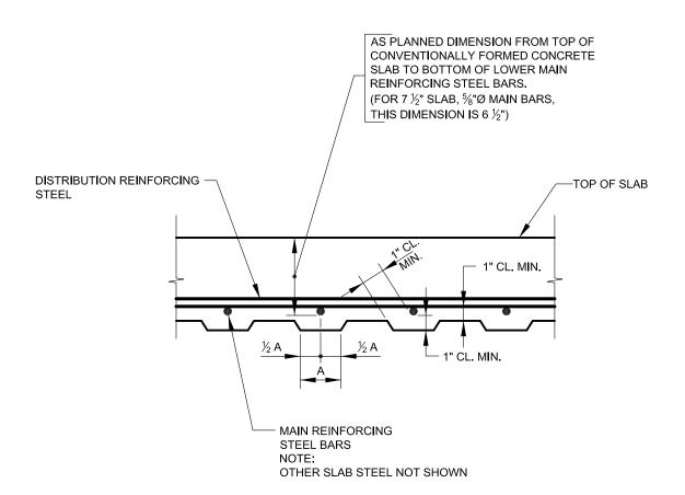
STEEL FORMS WHICH REMAIN IN PLACE SHALL BE THE PROPER GAUGE TO SUPPORT, WITHIN SPECIFIED DEFLECTIONS, THE SPECIFIED WEIGHTS FOR THE PARTICULAR SPAN INVOLVED AND SHALL BE ZINC-COATED ( GALVANIZED ) IN ACCORDANCE WITH ASTM SPECIFICATION A-653 AND A-924 COATING CLASS G-165. NOTE ALSO THAT NO FORM LESS THAN 20 GAUGE THICKNESS WILL BE ACCEPTED DUE TO DESIRE FOR DURABILITY.
