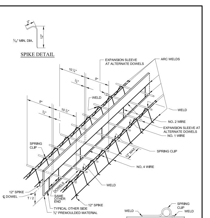
NOTES: SEE BC 572.21 FOR PAVEMENT THICKNESS AND THE REQUIRED DOWEL SIZES.
