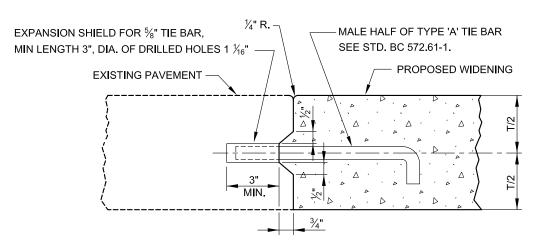
NOTE: THE TIE DEVICE TO BE PLACED 4' C.C. ALONG THE EDGE OF EXISTING PAVEMENT OR AS INDICATED ON THE PLANS OR WHERE AND IF DIRECTED BY THE ENGINEER.
