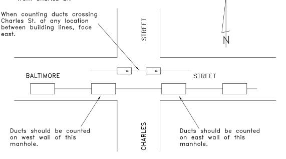
B. When identifying ducts in a North-South line, the count shall be made facing away from Baltimore St.
