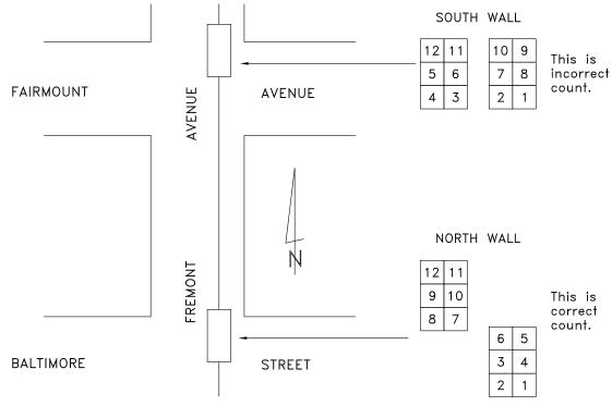
C. When a duct line leaves a manhole on either a north or south wall and enters a connecting manhole on the east or west wall, the general direction of the duct line shall be the deciding factor in determining the duct count.
