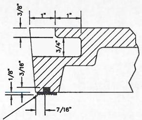
WATERTIGHT SEAL Machine Groove in Lid Seat for Oil-Resistant T-Gasket, Nitrile (60 Duro)
