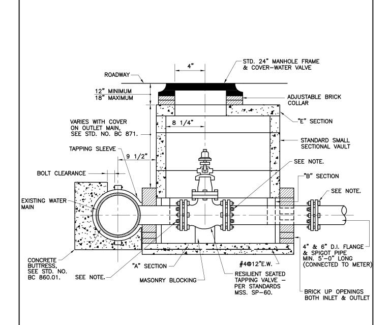
NOTE: ALL JOINTS MUST BE RESTRAINED BACK TO MAIN (ALL-THREAD RODS ARE NOT ACCEPTABLE).
