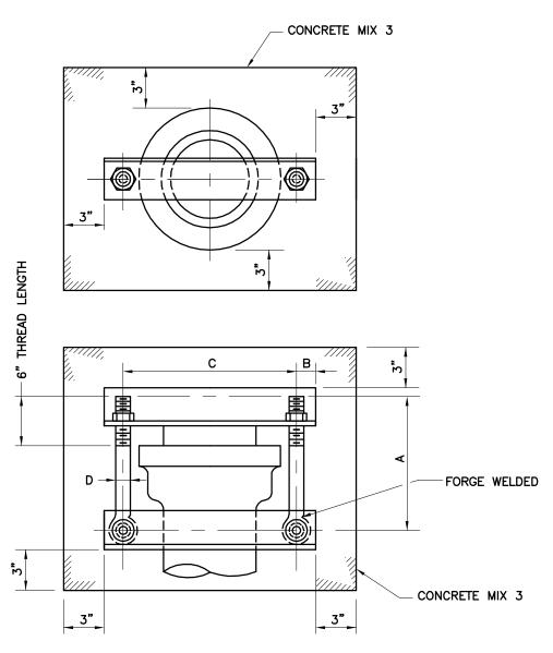
NOTE: MAKE HOLES IN ANGLE 1/8" LARGER THAN DIAMETER OF BOLT.
