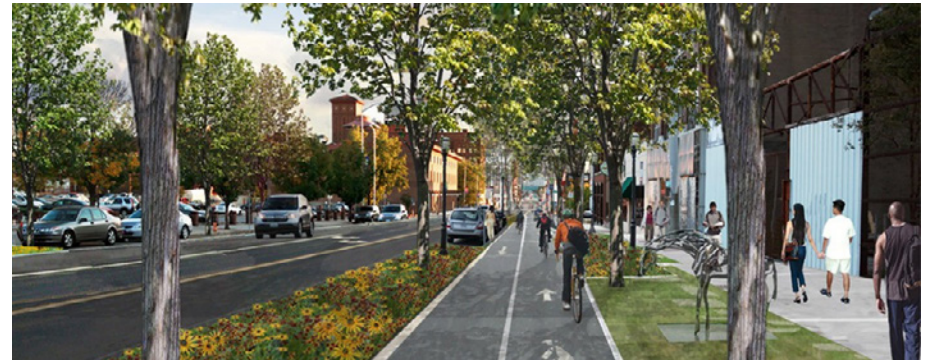
Figure 28: Two-way protected bike lane with landscaped buffers
