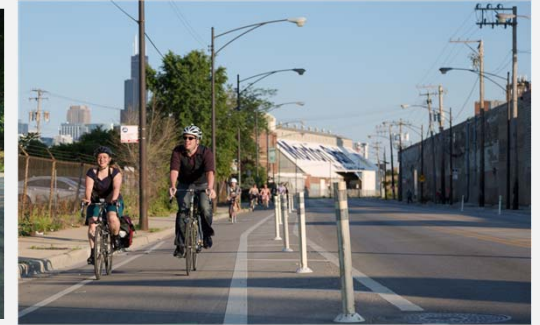
Water filled barrier demonstration. Flex post-delineated bike lane in Chicago. Photo: People for Bikes
