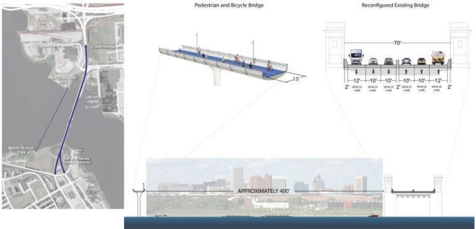
FIGURE 5-29: LAYOUT OF SEPARATE PEDESTRIAN / BICYCLE BRIDGE
