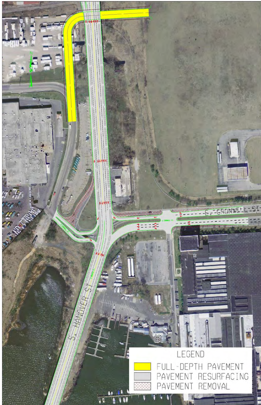
Figure 34 - Hanover Street at Cromwell Street Improvements (Right-In, Right-Out) and New Roadway Between West Covington and Port Covington Underneath Hanover Street (To Connect To Future Development)
