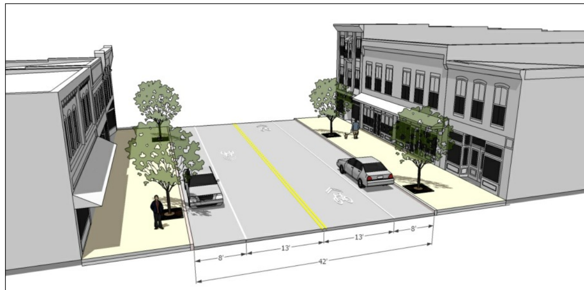
42' Neighborhood Mixed Use Street. Two way operation with addition of sharrows and additional street trees.
