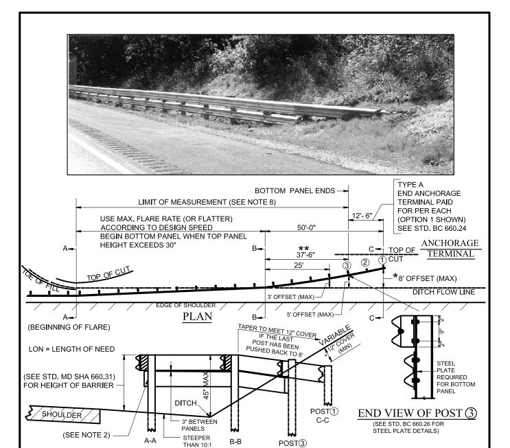
\* WHEN EARTH COVER OVER POST (1) EXCEEDS 12", END BOTTOM PANEL OFFSET DISTANCES 5' & 8' MAY BE LESSENED. HEIGHT OF THE PANEL MUST REMAIN CONSTANT RELATIVE TO DITCH ELEVATION.
