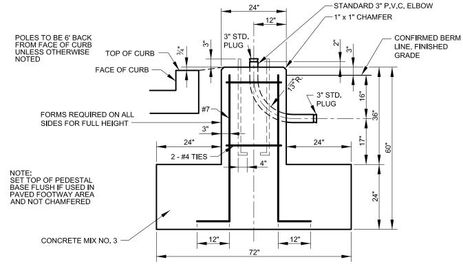
FOUNDATION BASE FOR POLES, UTILIZING MAST ARMS UP TO 18'
