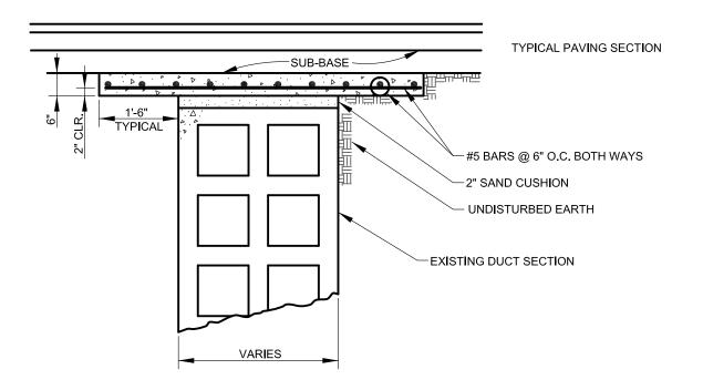
ALL CONCRETE TO BE MIX NO. 3. ALL REINFORCING STEEL TO CONFORM TO A.S.T.M. 615, GRADE 40  $\,$
