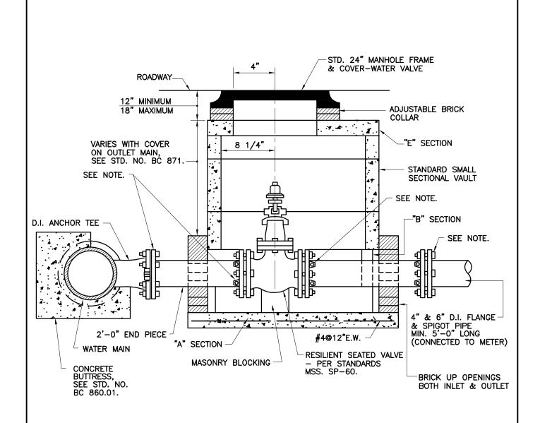
NOTE: ALL JOINTS MUST BE RESTRAINED BACK TO MAIN (ALL-THREAD RODS ARE NOT ACCEPTABLE).
