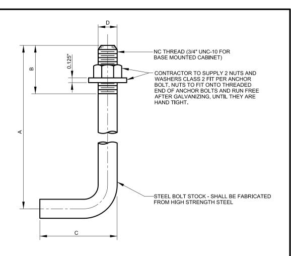
ANCHOR NUTS, BOLTS AND WASHERS SHALL BE HOT-DIPPED GALVANIZED IN ACCORDANCE WITH ASTM A 153. NUTS AND WASHERS SHALL MEET THE PHYSICAL AND CHEMICAL REQUIREMENTS OF ASTM A 307.
